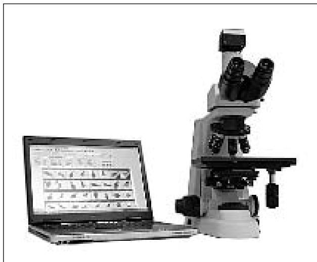
Figure 2. Computer and phase-contrast optical microscope.
